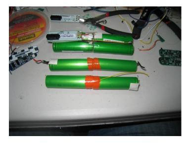
Then tape both rows together in such a way where you can solder one end together, to complete the connection of 4 cells in series. You will need to also add a piece of wire to that junction for later connecting to the protection board. On the other end, solder some heavier gauge wire to the positive and negative terminal, for later connection to the protection board. You can tell which end is positive, as it will have an indented ring around it.
