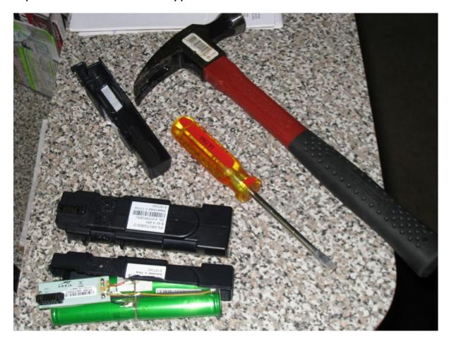
The batteries I used where in a plastic case. I removed all the stickers, and somewhat gently hit the case along the seam with a hammer. If done just right, the shell will fall apart, (I didn't even need the screw driver) and you get some yummy cells.
