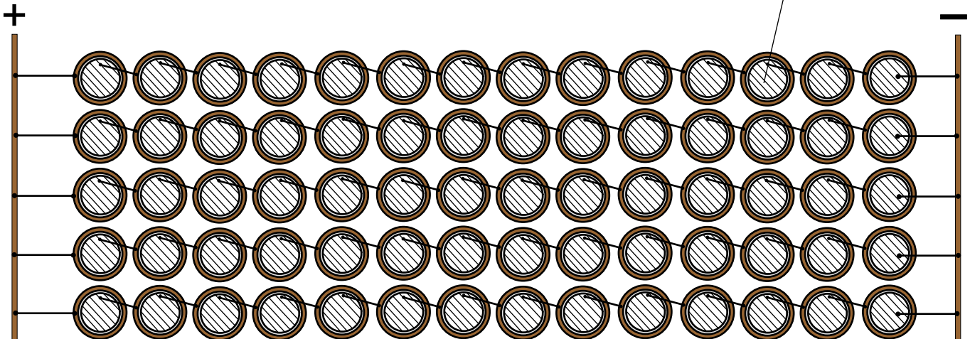
Example of a perfect Zinc rod copper pipe cell
