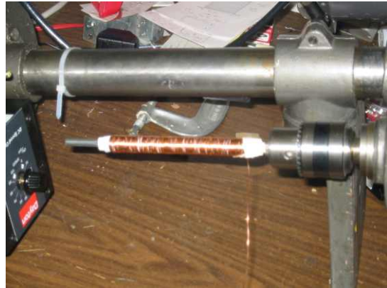
Small Drill press turned into a Coil Winder
